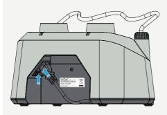
Plug the appropriate power cord into the power socket and switch the unit on using the On/Off switch.
