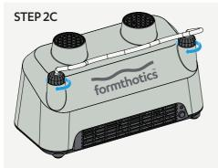
Once in the correct position, tighten the twist locks by rotating them clock-wise with a half turn.
